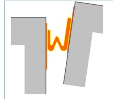
Fig. 5 - Jointspan FR installed in W shape after considerable seismic movement.
